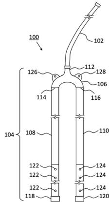
In particular, dry barrier-forming material is introduced into the tool at an initial flow velocity through a source conduit and is sent through a flow divider before exiting into two boreholes. The filling tool is placed in two boreholes and the dry barrier-forming material exits at a lower flow velocity than the initial velocity, while the tool is simultaneously raised, thereby solving the problem of stuck conduits and material blow-back.
